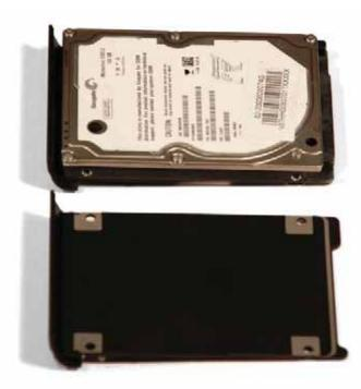
Turn the drive mount over as shown and align the HDD with the mounting holes for the screws.
