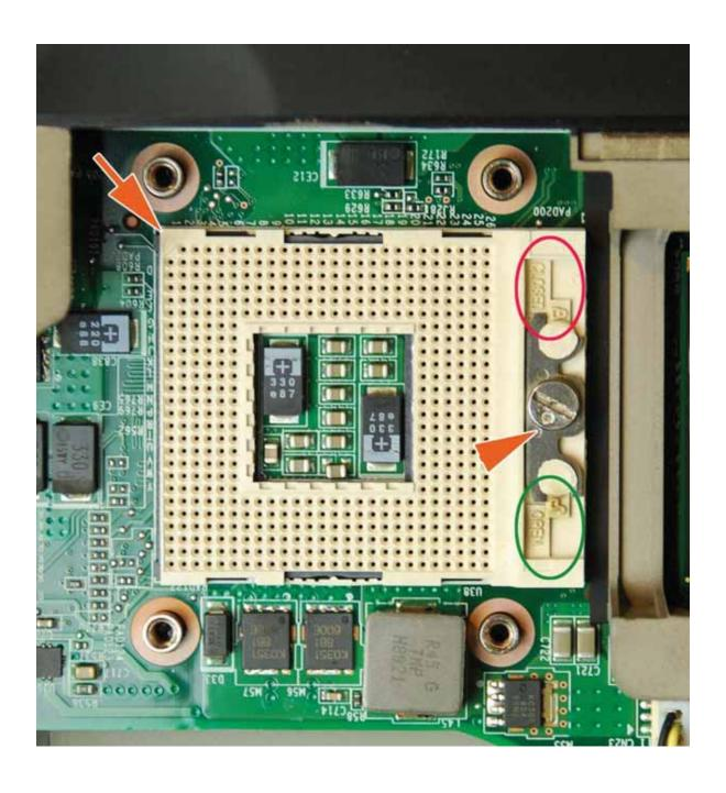
Note the golden triangle on the CPU package that needs to match the upper left corner In the orientation of the socket as shown in the pictures above. Also note the orientation of the locking screw with the notch facing the "closed" position.
