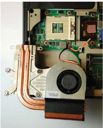
Locate the six screws (arrows) and unscrew them in the order indicated on the heatspreader (1-6). Carefully lift the cooling aggregate out of the cavity and place it on the side of the shell. It is not necessary to disconnect the fan from its power header on the motherboard (see arrow, right picture).
