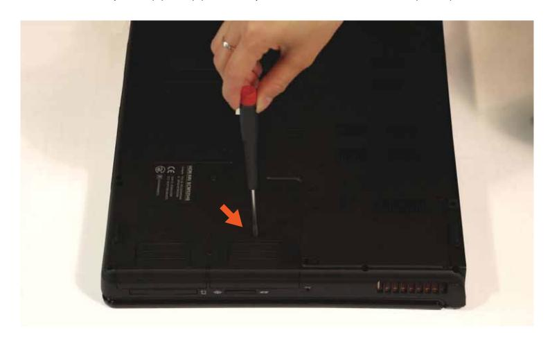
After removal of the screws, the drive mounts can be pulled from the laptop chassis.
