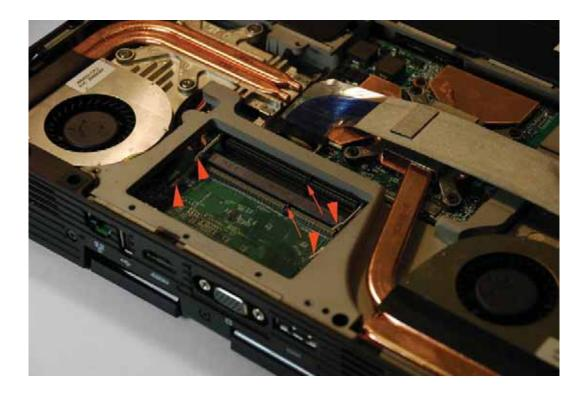
Please note that the two memory slots are "keyed" (arrows) to ensure correct orientation of the memory modules. Also note the retention clips (arrowheads) that will engage with the cutaway on the memory modules to secure them in place.
