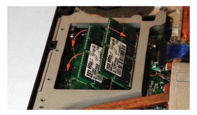
Position the memory modules in the slots and slightly tap them to ensure their full insertion. Then gently press the modules down starting with the lower module until they lie flat and engage with the retention clips as shown in the picture below.
